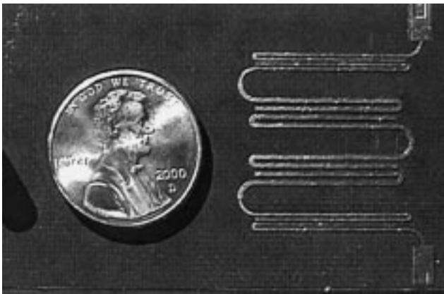
Fig. 12. Fabricated four-section maximally flat coupled four-line filter designed for a center frequency of 1.5 GHz.
